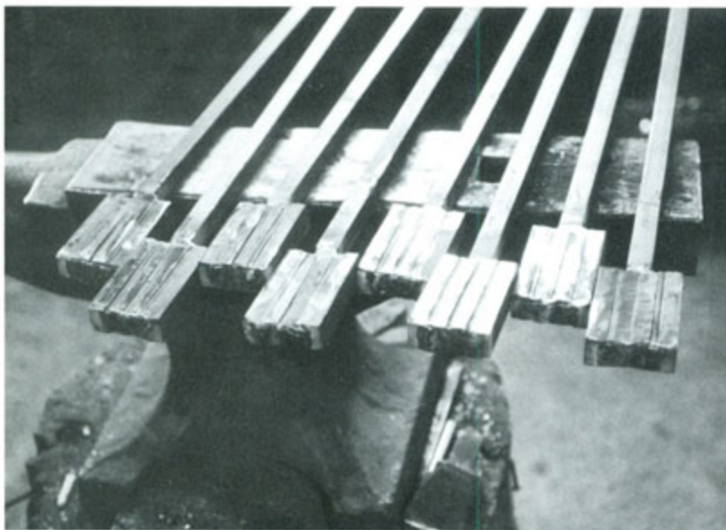
Eight billets before welding which will form the twisted core bars.
